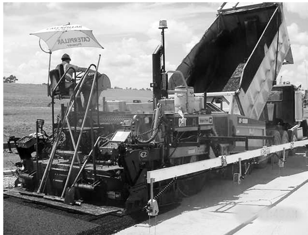
Figure 9-10 Long Mobile Grade Reference (Ski with Stringline)
